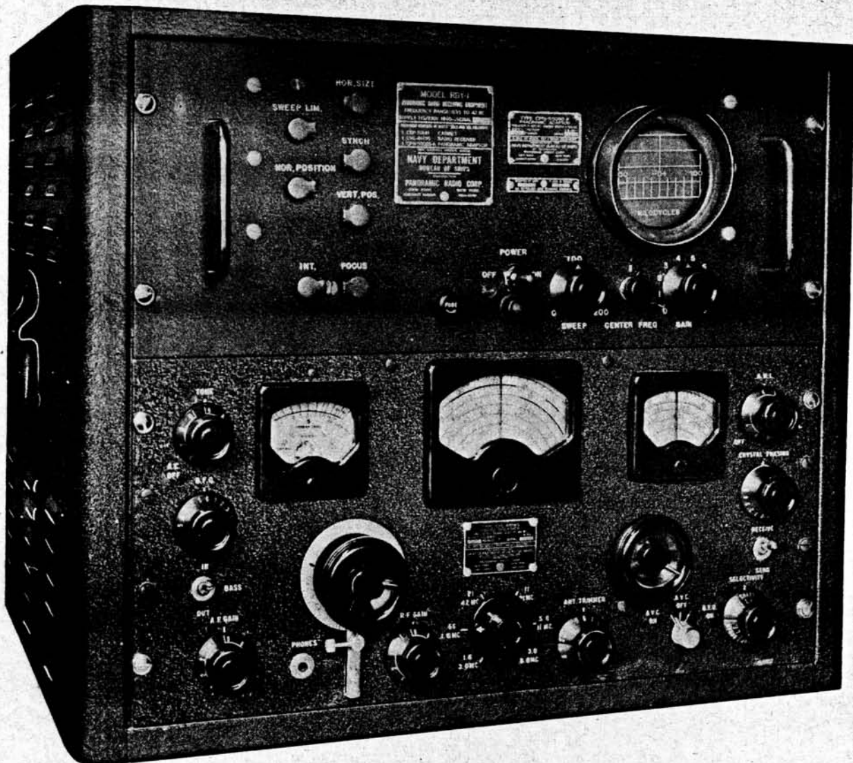
FIG.2 - PANORAMIC RECEIVING EQUIPMENT FRONT VIEW
